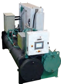
Oil Free Centrifugal HP Water to water heat pump Magnetic centrifugal compressor R134a Hot water up to 70°C R245fa Hot water up to 105°C Heating capacity from 700 to 1800 kW
