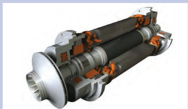
To eliminate mechanical-contact losses in the driveline, the YMC2 chiller utilises a permanent-magnet motor and active magnetic-bearing technology.
