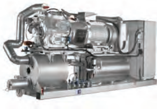
HeatPAC HPX recip Variable-Speed Drive Reciprocating compr. / R717 Hot water up to 90°C Heating capacity up to 600 kW at 40°C source
