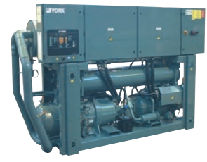
YLCS Water to water heat pump Twin screw comp. / R134a Hot water up to 70°C Heating cap.: 400 to 2000 kW
