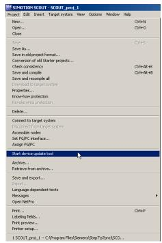
Figure 6-1 SIMOTION SCOUT - Starting the SIMOTION Device Update tool
