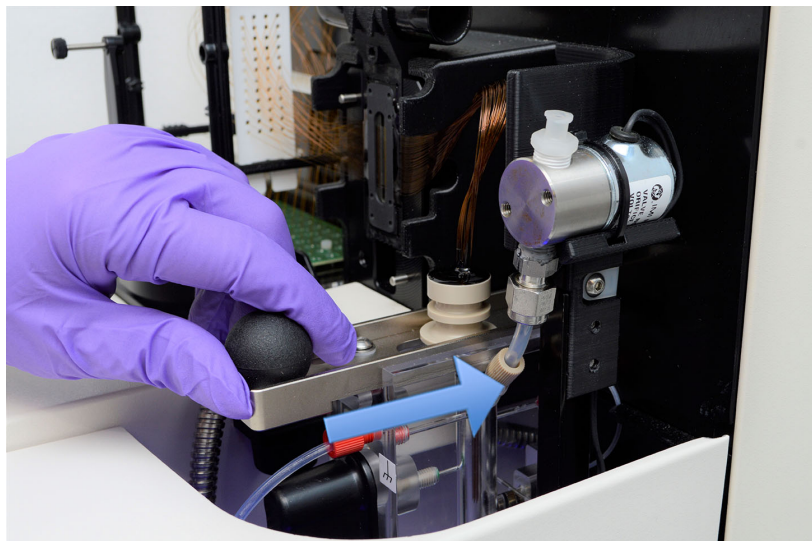
Figure 81 Instrument top compartment – capillary reservoir connector slide
