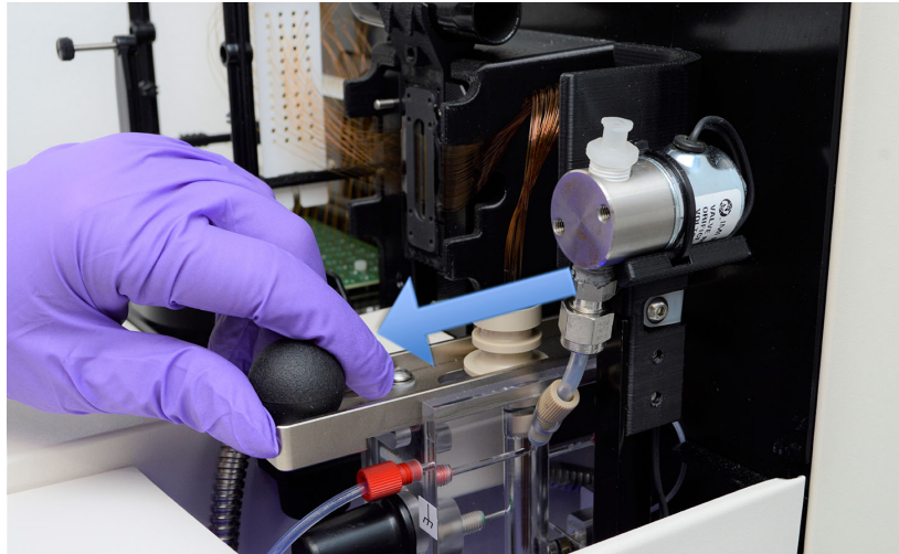
Figure 60 Instrument top compartment – capillary reservoir connector slide
