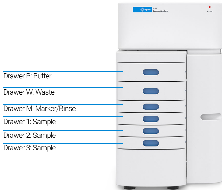
Figure 7 Instrument drawer positions
