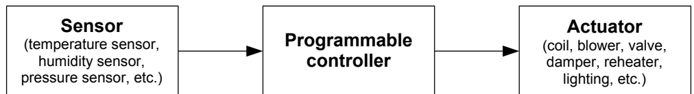
Figure 12. DDC controlled HVAC system operation.
