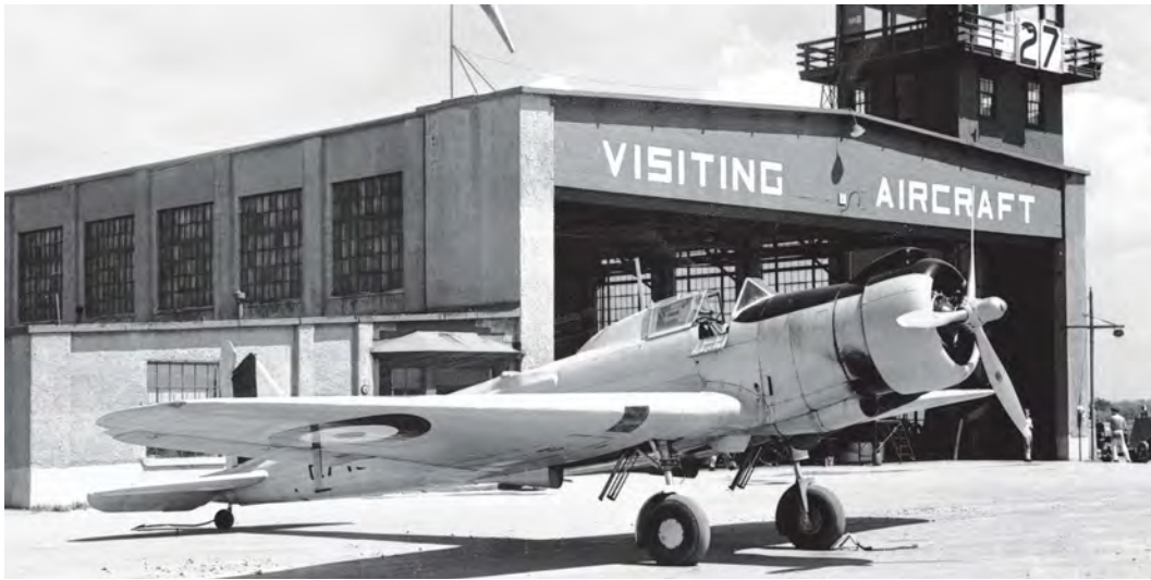
ABOVE: Just one Battle, R7439, was modified to MkII standard by Fairchild in Québec with a Wright R-1820 radial engine for trials in case Merlin supplies were disrupted. VIA LARRY MILBERRY
