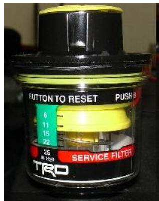
Partially Dirty Filter (Do Not Clean Now)
