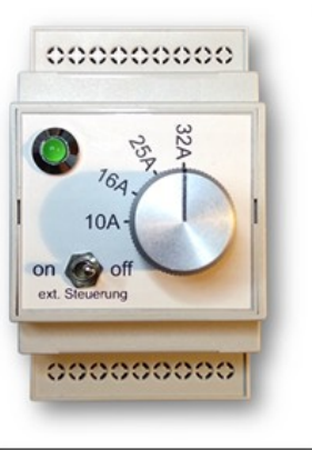
Picture 16: EVSE WB in custom box with 4position current switch
