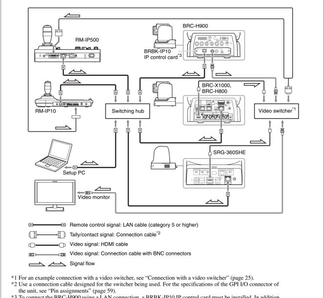
\*3 To connect the BRC-H900 using a LAN connection, a BRBK-IP10 IP control card must be installed. In addition, use an IP control card with firmware version 2.1 or later.
