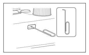
2 Pull the screw hole protective covers straight out.
