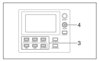
1 Set CONFIG >RM SETUP >AE CONFIG to MANUAL, IRIS Pri, GAIN Pri, or SHUTTER Pri in the RM menu.
