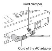
3 Thread the cord of the AC power adapter through the cord clamper, then close the lock.
