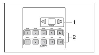
The number of camera numbers that can be assigned to cameras to control varies depending on the use of LAN connection or serial connection. The method of selecting the camera number also is different.
