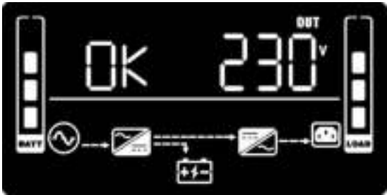
Figure 16: Display in normal mode
