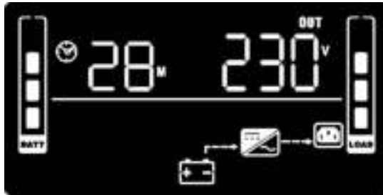
Figure 17: Battery mode display
