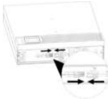
Figure 6: Connecting the battery
