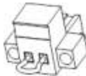
Figure 23: Emergency power off connector
