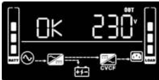
Figure 21: Display in frequency converter mode
