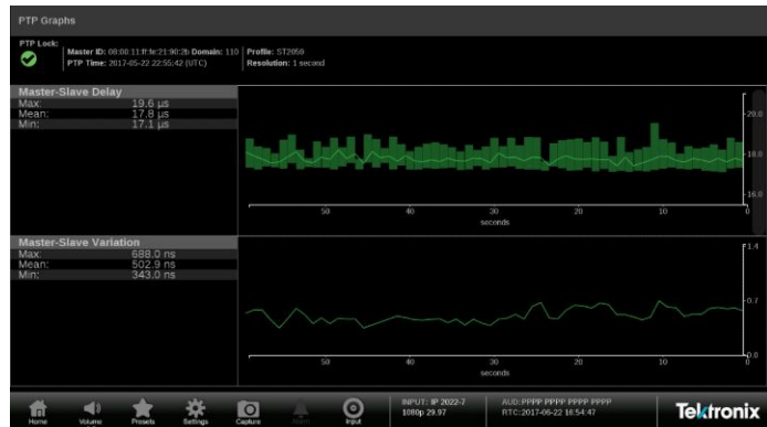
Master-Slave Delay and Master-Slave Variation graphs.
