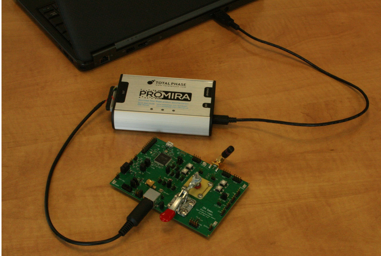
Figure 6. Connected Ezairo 7160 SL Hybrid Demonstrator Board, Windows PC, and Programming Box
