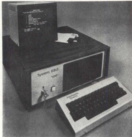
Line of PolyMorphic Systems 88 microcomputers includes System 8813 consisting of processor, mini-floppy drives, keyboard, video monitor, and system software
