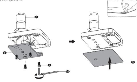
2. Remove clamp bolt from C-Clamp using Allen Key 6mm to . Place the Base noto the desk hole, and guide the Support Plate through the bolt. Tighten the bolt to the base for stability using Allen Key 6mm .
