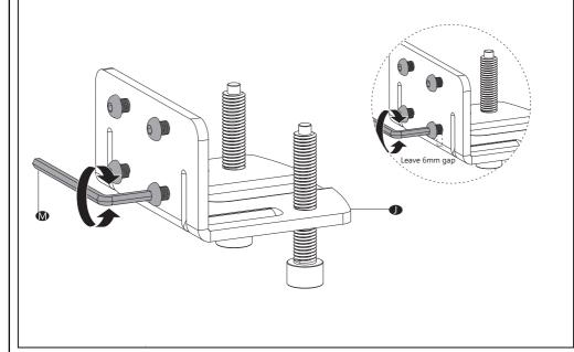
3. Hang the C-Clamp ① on the C-Clamp Brace ① to the preferred height according to your desk thickness and tighten using Allen Key 4mm ② . Place Support Plate ③ on top of clamp bolts.
