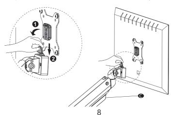
Press the Arm on horizontal level as image shown, adjust gas spring tension to your personal preference using Allen Key 6mm .
