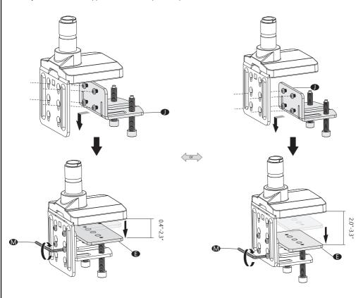
4. Position base on desktop and tighten clamp bolts evenly using Allen Key 6mm 🕦 . Attach Decor Cover 🕕 to back of C-Clamp Brace 🕕 .
