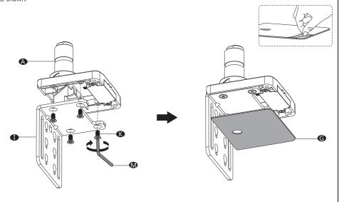
2. Loosen the Bolts on the C-Clamp  $\P$  using Allen Key 4mm  $\P$  .
