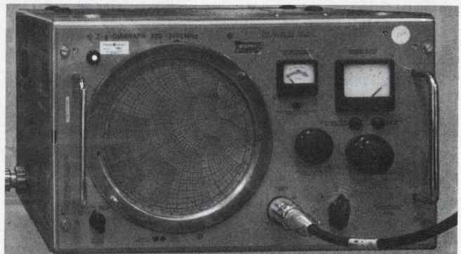
9. Rohde & Schwarz unit is most complex of all. Read-out is on a Smith chart and, though working at high frequencies, is limited to the input and output parameters. Transadmittance figures must be calculated by a complex and lengthy formula.
