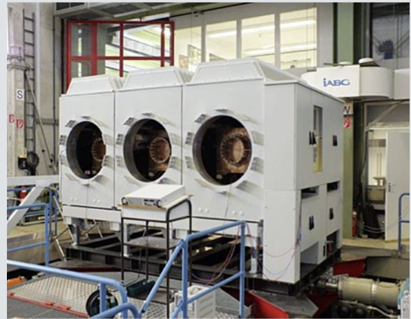
Fig. 54 HB3 switchgear during seismic testing
