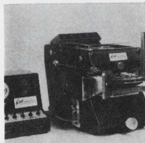
Screen printer model 1200-TT is a fully automatic machine tooled for high speed printing of conductor and resistor patterns on ceramic substrates. It screens fine lines—down to 0.003 in.—at rates up to 1,600 pieces per hour with \pm 0.001 in. repeatability, even on substrates with a 20% variation in thickness. Wells Electronics Inc., 1701 S. Main St., South Bend, Ind. 46623 [425]
