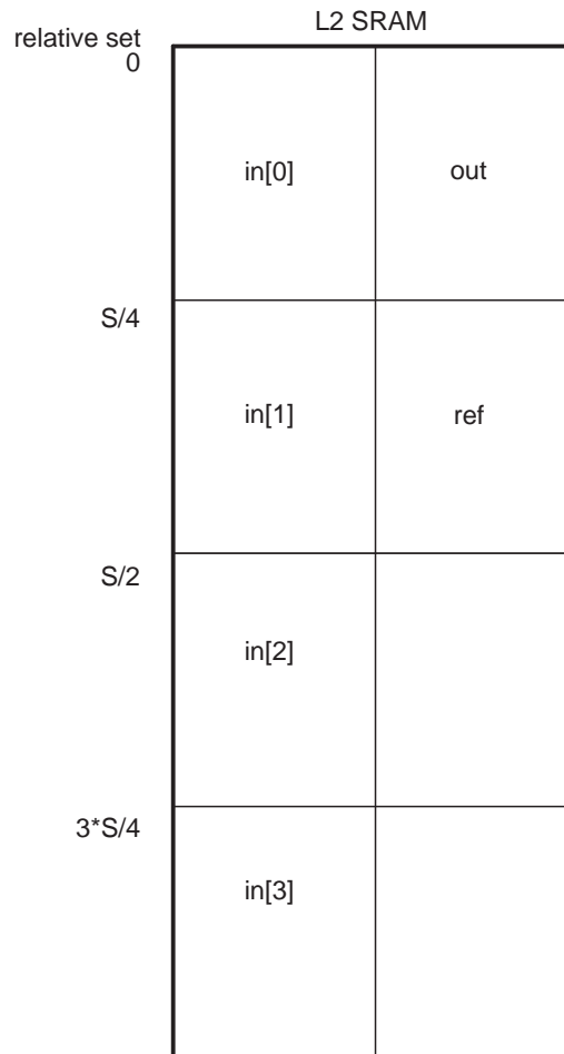
Figure 3-9. Memory Layout for Vecaddc/Dotprod Example
