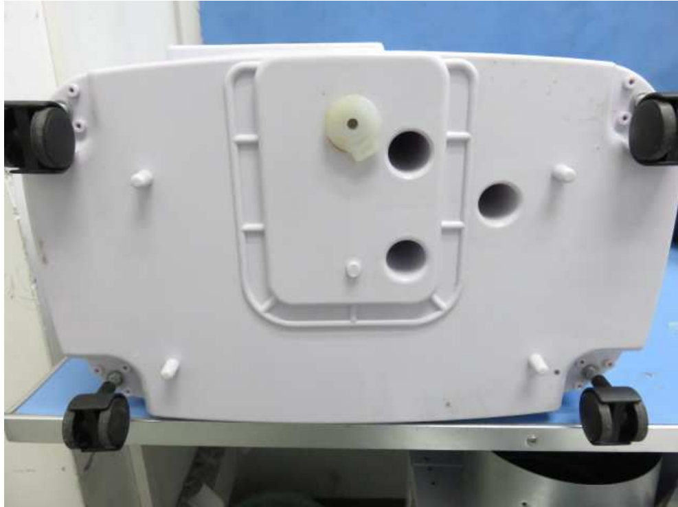
Bottom view (water drain hole diameter exceed 5mm)
