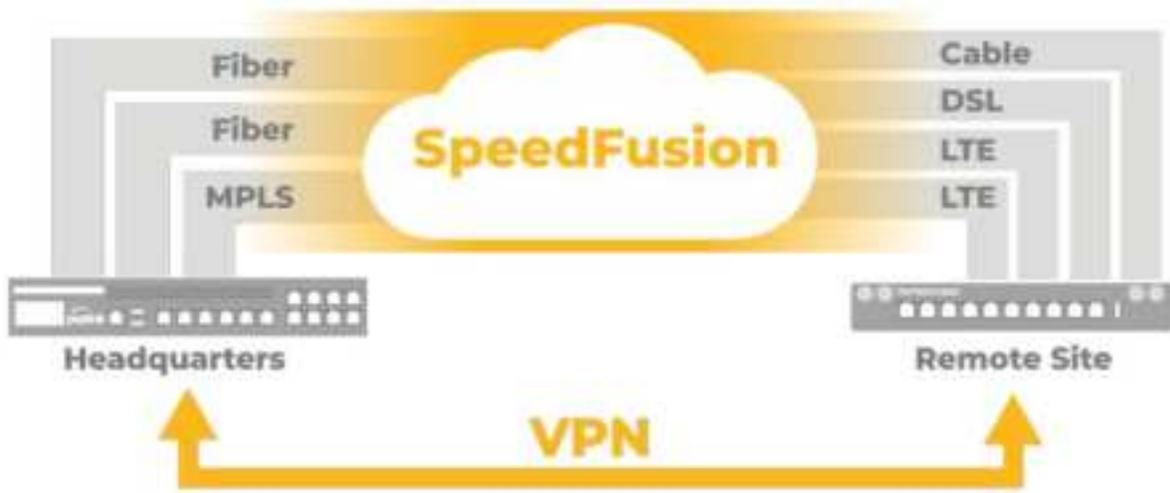
Peplink Balance SpeedFusion™ Bandwidth Bonding is our patented technology that enables our SD-WAN routers to bond multiple Internet connections to increase site-to-site bandwidth and reliability. SpeedFusion securely connects one or more branch offices to your company's main headquarters or to other branches. The data, voice, and video communications between these locations are kept confidential across the public Internet.
