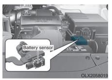
The battery sensor is deactivated, when the battery is disconnected from the negative pole for maintenance purpose.
