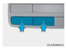
2. To turn off the 3rd row air conditioning control system, press the 3rd row air conditioning ON/OFF button once more located on the front climate control panel or set the fan speed to the OFF position with the 3rd row fan speed switch (indicator light on the ON/OFF
