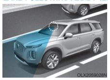
The Lane Following Assist (LFA) system helps detect lane markers on the road with a front view camera at the front windshield, and assists the driver's steering to help keep the vehicle between lanes.
