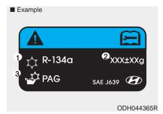
The actual Air Conditioning refrigerant label in the vehicle may differ from the illustration.
