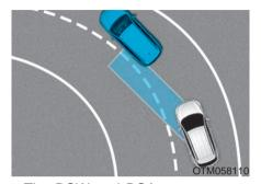
The BCW and BCA systems may not operate properly when driving on a curved road. In certain instances, the system may recognize a vehicle in the same lane. Always pay attention to road and driving conditions, while driving.
