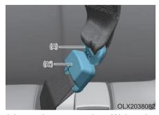
Insert the tongue plate (A) into the buckle (A') until an audible "click" is heard, indicating the latch is locked. Make sure the belt is not twisted.
