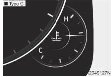
This gauge indicates the temperature of the engine coolant when the ignition switch is in the ON position.
