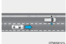
The Lane Change Assist feature will alert you when it detects a vehicle is approaching in an adjacent lane at a high rate of speed. If the driver activates the turn signal when the system detects an oncoming vehicle, the system sounds an audible alert.
