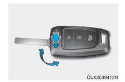
If the remote key does not operate normally, you can lock or unlock the driver's door by using the mechanical key.
