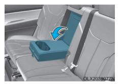
The armrest is located in the center of the rear seat. Use the strap in the center of the armrest to pull it down.
