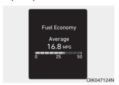
The trip computer mode displays information related to vehicle driving parameters including fuel economy, tripmeter information and vehicle speed.
