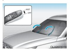
This vehicle has a "hidden" wiper design which means that the wipers cannot be lifted when they are in their bottom resting position.
