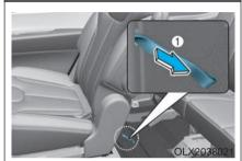
If the walk-in switch does not work, pull the strap (1) located on the lower left side of the seat. Then you can move the 2nd row seat forward
