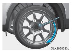
14. Use the wheel lug nut wrench to tighten the lug nuts in the order shown. Double-check each lug nut until they are tight. After changing tires, have an authorized HYUNDAI dealer tighten the lug nuts to their proper torque as soon as possible. The wheel lug nut should be tightened to 79~94 lbf-ft (11~13 kgf-m).
