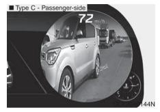
BVM (Blind-spot View Monitor) system displays the driver-side or passenger-side rear areas in the cluster when the system is activated.
