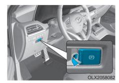
To apply the EPB (Electronic Parking Brake):
