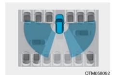
The Rear Cross-Traffic Collision Warning (RCCW) system uses radar sensors to monitor the approaching cross traffic from the left and right side of the vehicle when your vehicle is in reverse.
