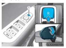
When you move the shift button to the R (Reverse) position, the side view mirror(s) will rotate downwards to aid with driving in reverse. The position of the side view mirror switch (1) determines whether or not the mirrors will move:
