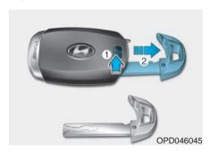
To remove the mechanical key from the smart key FOB, slide the release lever in the direction of the arrow (1) and then pull the mechanical key (2) outward.
