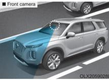
In order for the FCA system to operate properly, always make sure the sensor cover or sensor is clean and free of dirt, snow, and debris.
