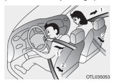
Your vehicle is equipped with driver's and front passenger's Pre-tensioner Seat Belts (Retractor Pretensioner).
