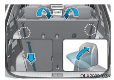
The headrest will fold down automatically when folding the seatback.
