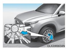
Insert the tool (1, if equipped) into the hole and pull out the wheel cover.
