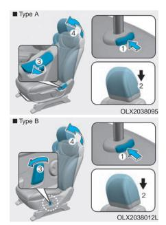
To reinstall the head restraint:
