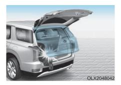
During power opening and closing if the power liftgate is blocked by an object or part of the body, the power liftgate may be able to detect the resistance.
