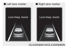
1. A visual warning appears on the cluster LCD display. Either the left lane marker or the right lane marker in the cluster LCD display will blink depending on which direction the vehicle is veering. Also, the steering wheel will vibrate.
