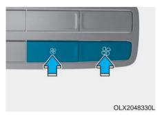
The fan speed can be set to the desired speed by pushing the fan speed control button. The higher the fan speed is, the more air is delivered.
