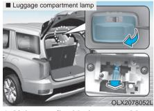
Using a flat-blade screwdriver, gently pry the lens from the interior lamp housing.
