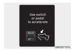
Use switch or pedal to accelerate While the Smart Cruise Control (SCC) system is operating, your vehicle stops behind the vehicle in front when it stops. The message shown above is displayed on the cluster within 3 seconds after the stop and the system will be in the standby position.
