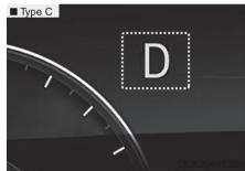
This indicator displays the gear position of the shift button.
