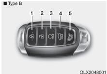
Your HYUNDAI uses a Smart Key, which you can use to lock or unlock the driver and passenger doors or the rear liftgate.
