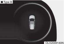
If the driver turns off the engine when the sunroof is not fully closed, the warning chime will sound for approximately 3 seconds and the sunroof open warning will appear on the cluster LCD display.  If the driver turns off the engine and opens the door when the sunroof is not fully closed, the sunroof open warning will appear on the cluster LCD display until the door is closed or the sunroof is fully closed.
