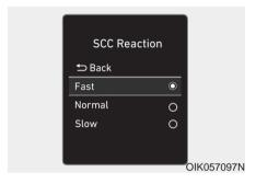
The sensitivity of vehicle speed when following the front vehicle to maintain the set distance can be adjusted. Go to the 'User Settings  $\rightarrow$  Driver Assistance  $\rightarrow$  SCC Reaction  $\rightarrow$  Fast/Normal/Slow' on the LCD display. You may select one of the three stages you prefer.
