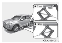
8. Place the jack at the designated jacking position under the frame closest to the tire you are changing. The jacking positions are plates welded to the frame with two notches. Never jack at any other position or part of the vehicle. Doing so may damage the
