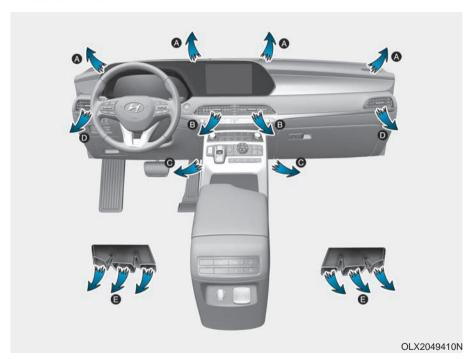
The mode selection button controls the direction of the air flow through the ventilation system. Air can be directed to the floor, dashboard outlets, or windshield. Five symbols are used to represent Face, Bi-Level, Floor, Floor-Defrost and Defrost air position.
