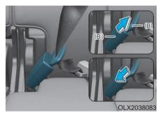
Pull out the tongue plate (B) from the pocket. Pull the tongue plate (B) and insert it into the buckle (B') until an audible "click" is heard, indicating the latch is locked. Make sure the belt is not twisted.
