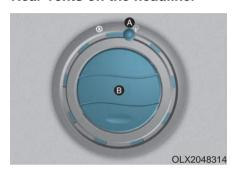
The rear passengers can adjust the direction of air flow from the rear vents on the headliner.
