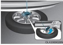
Draw out the retainer guide (1) through the center hole of the spare tire. To store the spare tire:
