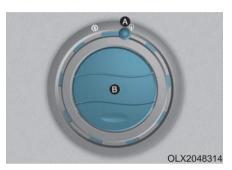
The rear passengers can adjust the direction of air flow from the rear vents on the headliner.
