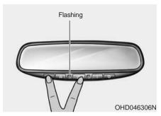
1. When programming the buttons for the first time, press and hold the left and center buttons (全, 金) simultaneously for approximately 20 seconds until the indicator light begins to flash. (This procedure erases the factory-set default codes. Do not perform this step to program additional hand-held transmitters.)
