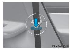
3. Locate the seatbelt webbing in the guide before folding down the seatback to avoid the seatbelt system interfering with the seatback.
