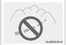
Do not drive across the contour of steep hills. A slight change in the wheel angle can destabilize the vehicle, or a stable vehicle may lose stability if the vehicle stops its forward motion. Your vehicle may roll over and lead to a serious injury or death.
