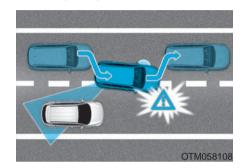
The Blind-Spot Collision-Avoidance Assist (BCA) system helps detect the front lane through the camera installed on the upper front windshield and helps detect the side/rear areas through radar sensors.
