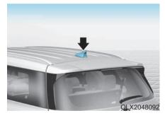
The shark fin antenna will receive the AM, FM broadcast signals and transmit data.
