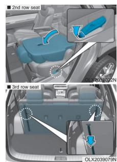
Pull up the seatback recline lever, then fold the seat toward the front of the vehicle.
