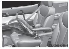
A rearward-facing child seat provides restraint with the seating surface against the back of the child. The harness system holds the child in place, and in an accident, acts to keep the child positioned in the seat and reduce the stress to the neck and spinal cord.
