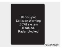
Blind-Spot Collision Warning (BCW) system disabled. Radar blocked
