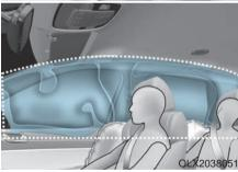
Curtain air bags are located along both sides of the roof rails above the front and rear doors.
