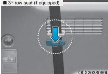
Routing the seat belt webbing through the rear seat belt guides will help keep the belts from being trapped behind or under the seats.
