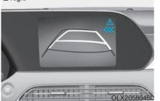
If the risk of collision is detected while the RCCW is generated, brake is controlled. The instrument cluster will inform the driver of the brake control. If the rear view monitor system is in activation, a message will also appear on the infotainment screen.
