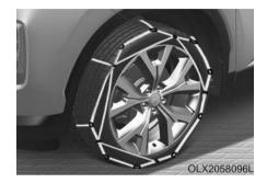
The mounting of some types of tire chains may cause damage to the tire. Therefore the use of snow tires is preferred over the use of tire chains.
