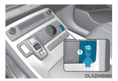
The Surround View Monitoring system can assist in parking by allowing the driver to see around the vehicle. Push the button (1, indicator ON) to operate the system. To cancel the system, push the button again (1, indicator OFF).
