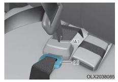
2. To retract the rear center seatbelt, insert the tongue plate into the web release hole (A'). Pull up on the seat belt web and allow the webbing to retract automatically. Insert the tongue plate (A) into the hole on the belt assembly cover.
