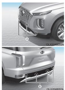
[A]: Front Sensor, [B]: Rear Sensor
