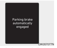
Parking brake automatically engaged
