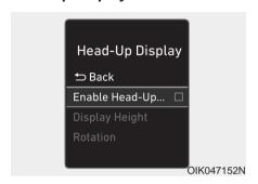
To activate the head up display, select 'Head-UP Display' on the User Settings mode on the instrument cluster LCD display.
