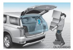
On vehicles equipped with a smart key, the liftgate can be opened with hands-free activation using the Smart Liftgate system.
