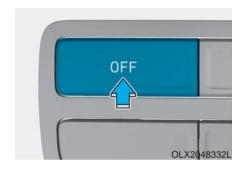
Push the OFF button to turn the rear climate control system off.
