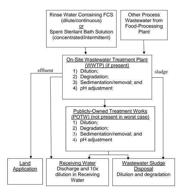
This diagram shows many of the common treatment steps that may be employed by food processing facilities using the FCS under the applications covered by this FCN. Direct discharge from the WWTP would result in higher concentrations of FCS in the environment than the indirect discharge from the POTW. Thus, we have assumed in determining the worst-case
