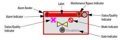
Each graphic symbol includes a touch field over it that opens the object's faceplate. In addition, there is a tooltip on the graphic symbol that displays the object's configured tag and description.
