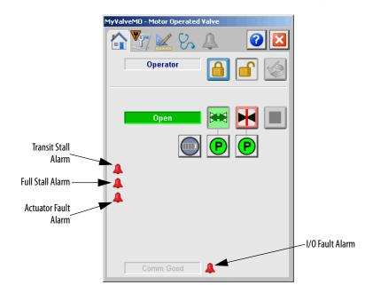
Alarm indicators appear on the Operator tab when a corresponding alarm occurs.
