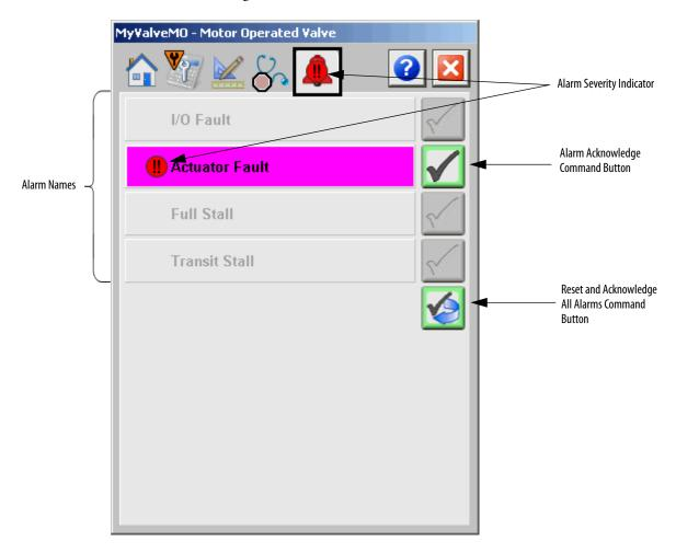
Click an alarm name to open the P\_Alarm faceplate for that alarm. From the P\_Alarm faceplate, you can configure and perform additional operations on the alarm.
