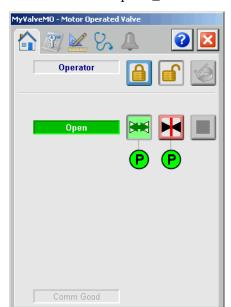
In the Operator faceplate example that follows, the P\_ValveMO instruction does not have associated Open P\_Perm, Close P\_Perm, or P\_ValveStats objects.
