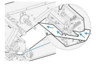
11. Pull out approximately 40 cm (15 in) of labels and remove the labels from the liner.
