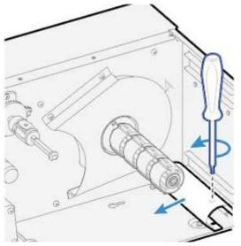
6. Remove the tear bar from the print unit and replace it with the guide plate.
