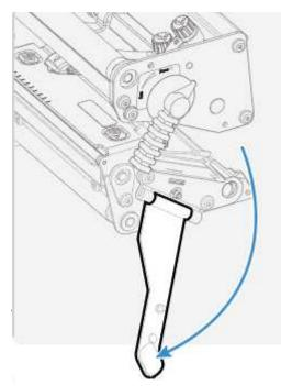
4. Raise the printhead by turning the printhead lift lever counter-clockwise.
