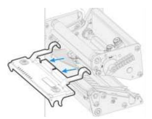
9. Connect the two cables to the replacement printhead.
