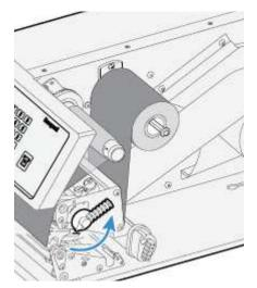
4. Remove any empty core from the media supply hub.
