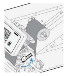
5. Remove any empty core from the media supply hub.
