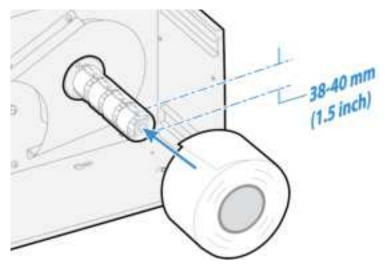
8. Route the media under the slack absorber and forward toward the print mechanism. The slack absorber can be rotated for better access and then snap-locked in open position.
