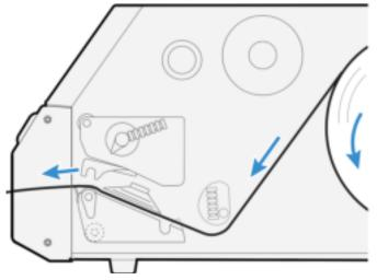
10. Lower the printhead by turning the printhead lift lever clockwise.
