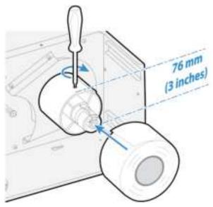
7. Fit a new roll of media on the supply post and push the roll in as far as it will go.
