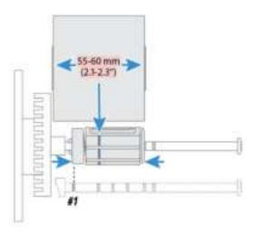
• If your ribbon is 88 to 90 mm (3.5 in) wide, compress the ribbon supply bobbin and move it so it snaps into the second groove.
