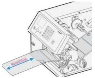
12. Route the liner around the tear bar and back under the print unit.
