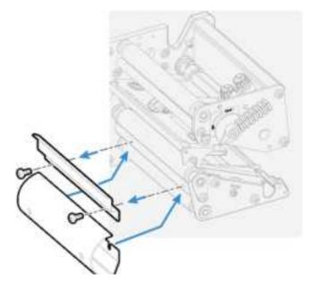
7. If you are using a media roll with a 76 mm (3 in) core, fit an adapter on the media supply hub.
