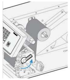
5. If necessary, remove the empty core from the media supply roll post.
