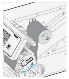
5. Pull out the red clip on the liner take-up hub and dispose of any wound-up liner.
