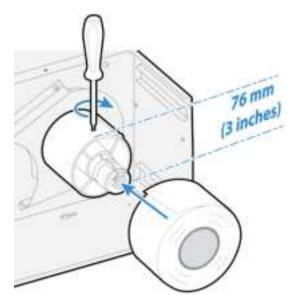
7. Fit a new roll of media onto the media supply hub and push the roll in as far as it will go.
