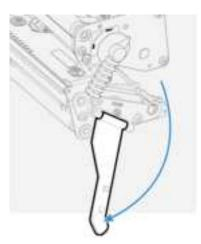
4. Turn the printhead lift lever counterclockwise to raise the printhead.
