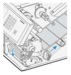
13. Secure the liner to the take-up hub with the red clip and rotate the hub until the media is pulled tight.
