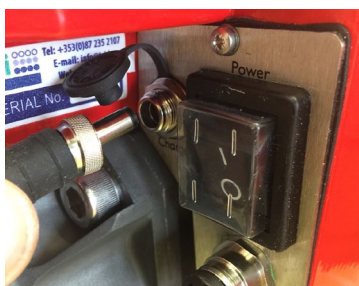
Fig. 5.1(a) Flowmaster battery charger socket (power panel)
