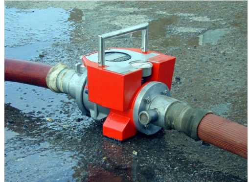
Fig. 4.4 Inline use of Flowmaster. Photograph courtesy of Essex County Fire and Rescue Service
