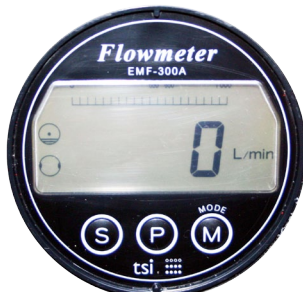
Fig. 3.3 Flow meter display when ready for flow measurement and there is no water in the pipe. Note the flashing symbols on the left side of the flowmeter gauge
