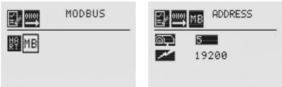
Figure 182. Modbus Configuration Display screen
