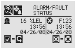
Figure 162. Alarm/Fault Status screen
