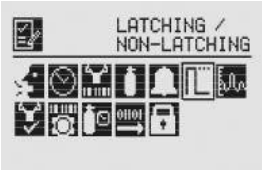
Figure 93. Alarm Latching/Non-Latching screen
