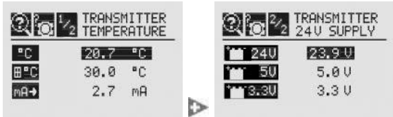
Figure 169. Transmitter Temperature and Supply Voltage screens
