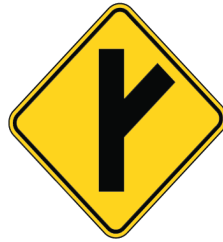
Side road enters highway ahead at an angle.
