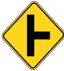
Side road enters highway ahead.
