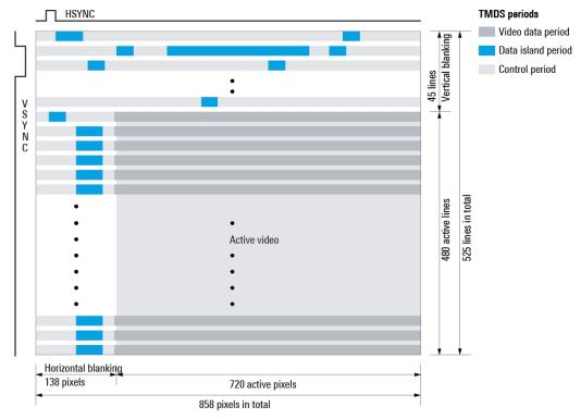
Fig. 2-3: Example of a TMDS frame structure in 720x480 format.
