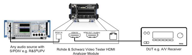
Fig. 4-10: Testing the ARC using the R&S<sup>®</sup>VTC/VTE/VTS.
