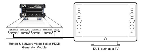
Fig. 5-2: Typical test setup for testing an HDMI sink.
