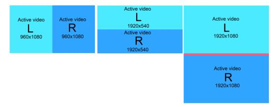
Fig. 2-4: The various 3D formats: Side-by-side (left), top-and-bottom (middle) and frame packing (right).
