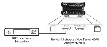
Fig. 4-1: Typical test setup for testing an HDMI source.
