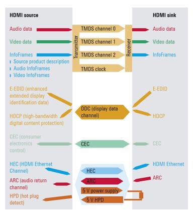
Fig. 2-1: Schematic illustration of the data transfer between the HDMI source and the HDMI sink.
