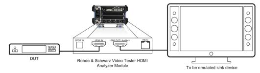
Fig. 4-12: Test setup for emulating a connected sink.
