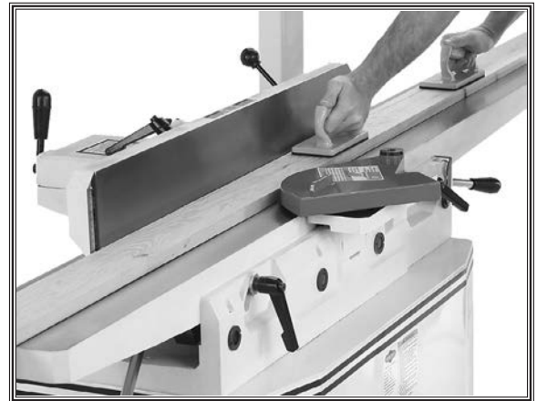
Figure 30. Typical surface planing operation.
