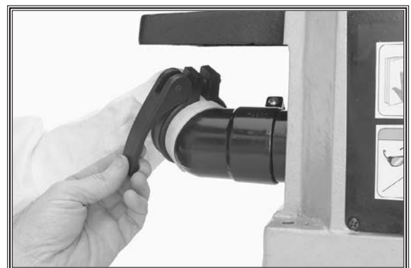
Figure 17. Attaching the dust collection bag.
