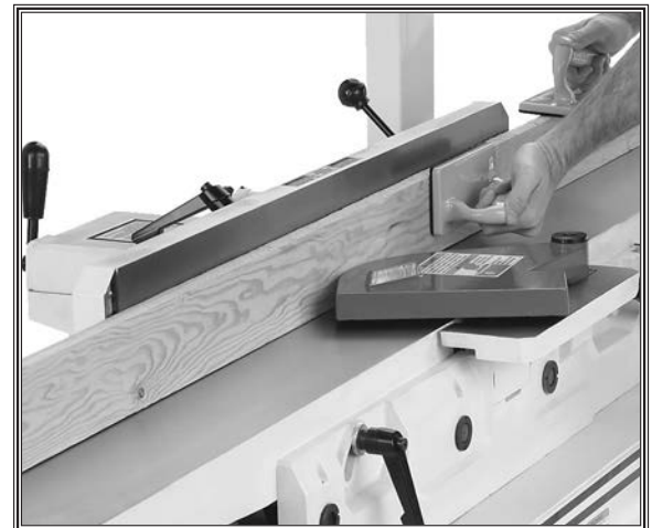
Figure 33. Typical edge jointing operation.
