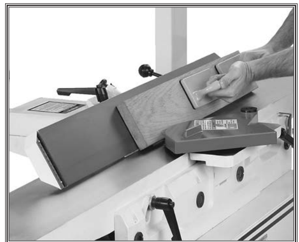
Figure 35. Typical bevel cutting operation.
