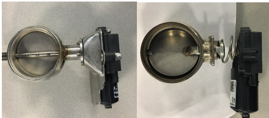
Fig. 1: Exhaust flow control valve with shield(left) and without shield (right: showing spring link)
