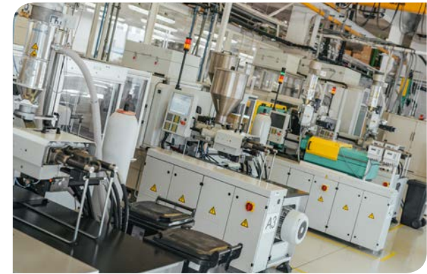
Production Room with Injection Moulding Machines
