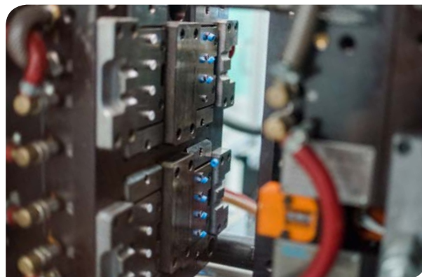
2-Component Moulding for XT Screw Caps
