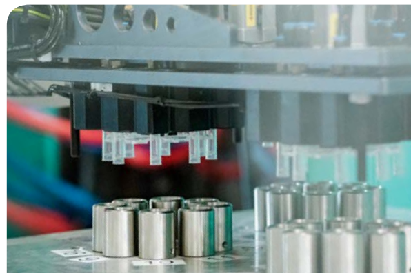
Transfer of Tubes from Injection Moulding Machine to Clean Room – Single Cavity Quality Control by an Automated Gripper Arm
