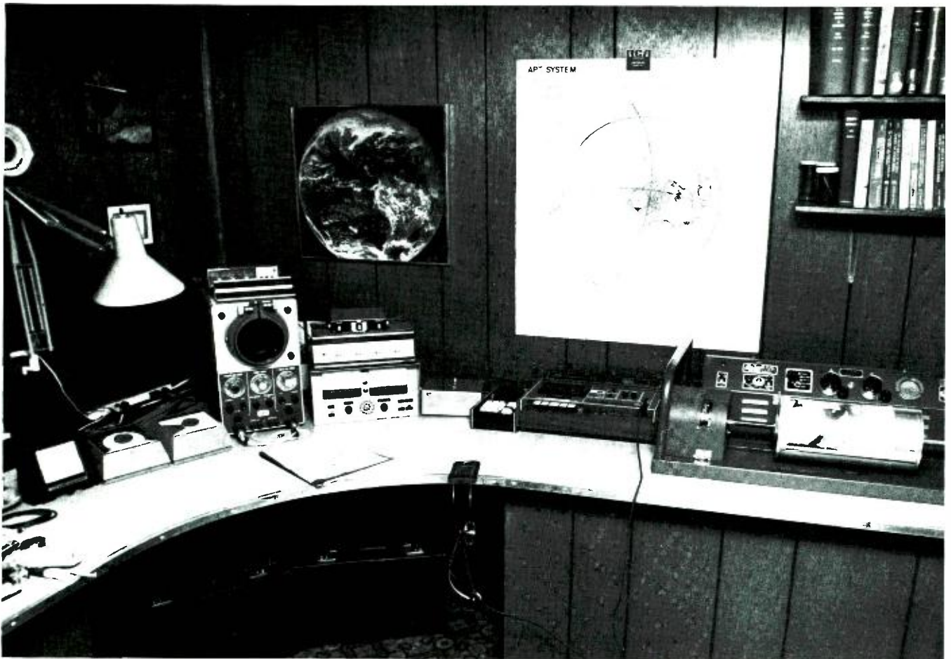
Author's complete APT weather satellite ground station in Mt. Laurel, N.J.
