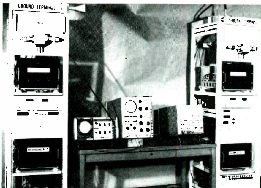
Fig. 9 — RPV/AJ communication system.
