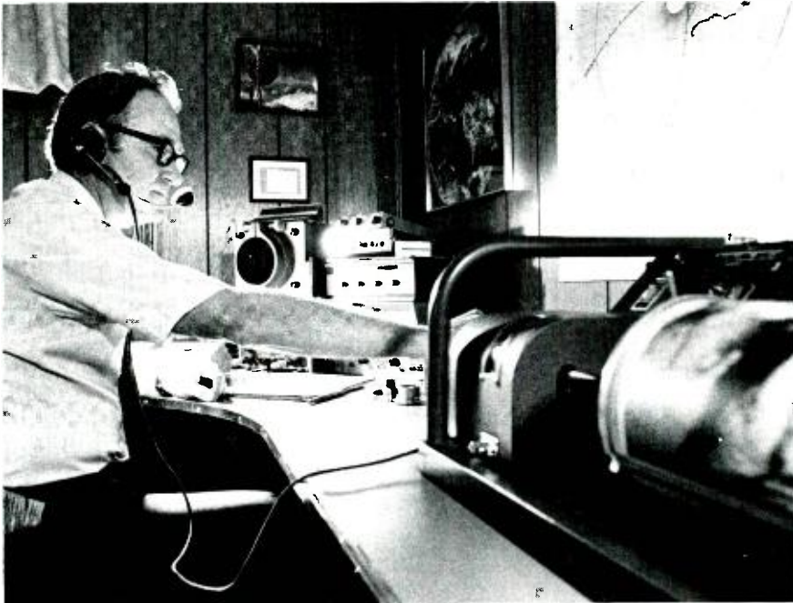
Lou Follet producing a photographic image from data transmitted from a NOAA-4 satellite pass. Cloud-cover photo (8 x 10-inch) is made on TXC-1 facsimile unit in foreground.
