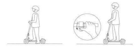
3. When stepping on both legs, press the accelerate button.
