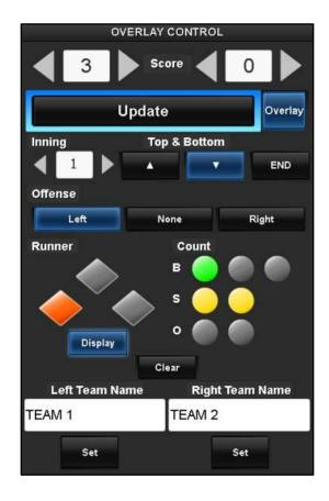
The **Clear** button is used to clear the **Runner** and **Count** display, for when the teams switch from offense to defense at the top or middle of an inning. The **Display** button below the diamond base indicators causes the **Runner** and **Count** to be displayed. When it is blue, they are displayed in the overlay.
