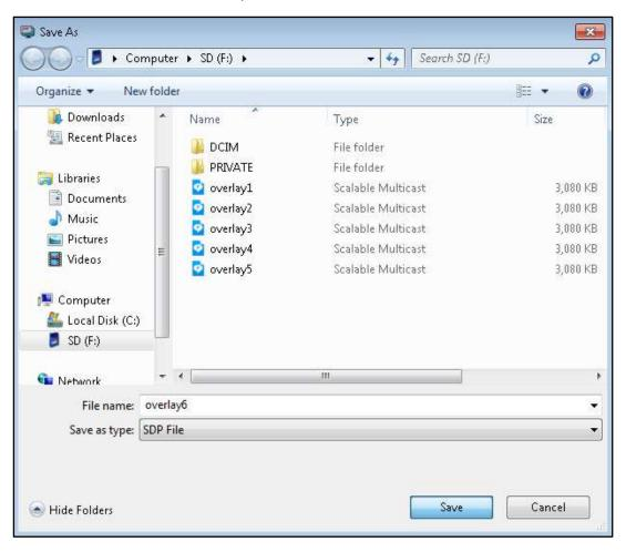
7) To import the overlay into the camera, copy the .sdp file onto the root directory on the Sd card (if you haven't already saved it there). Insert the card into one of the Sd card slots on the camera and access the Menu. 8) Enter the **Overlay Settings** sub menu and then choose **Import User Layout**.
