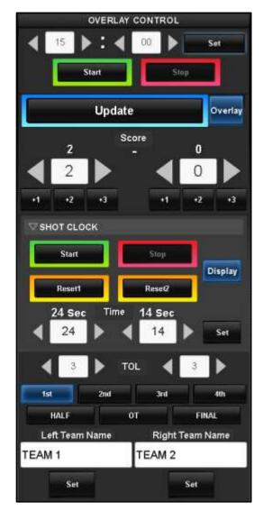
causes shot clock 1 to be displayed. Shot clock 2 is displayed after pressing **Reset 2**. The time selected for the shot clock may be configured by entering a number or by using the arrows. Once the needed time is displayed, pressing or clicking on the **Set** button configures that clock going forward.
