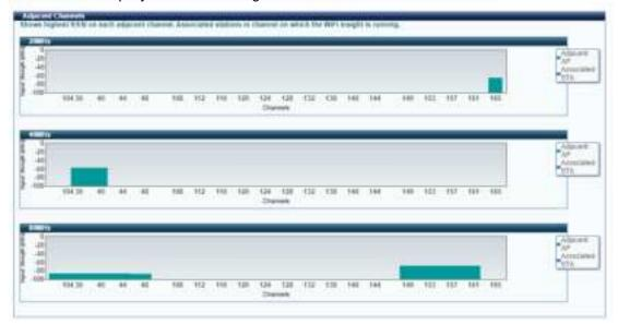
Shows the channel distribution and the possible interference caused for each AP.
