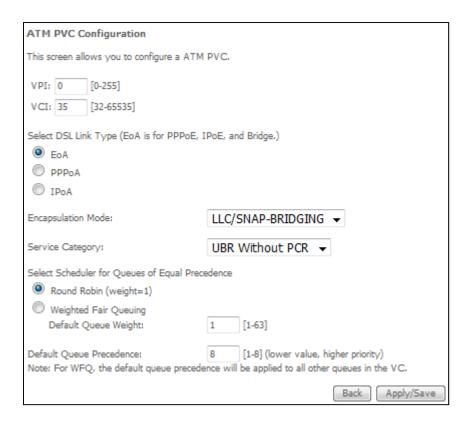
There are many settings here including: VPI/VCI, DSL Link Type, Encapsulation Mode, Service Category and Queue Weight. Here are the available encapsulations for each xDSL Link Type:
