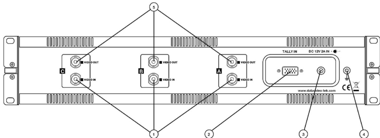
1. Each monitor has a composite video input, with a loop-through output (5). The video input can be PAL or NTSC, the TLM-433 will automatically detect the video standard.
