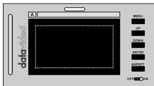
**Backlight** - There are 3 preset backlight levels which control the overall brightness of the monitor output. In a bright area it may be necessary to set Level 3 for maximum output, whereas in subdued lighting Level 1 will be adequate.
