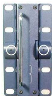
On either side of the TLM-433 are small Allen Key screw tension adjustments. These alter the tension on the pivoting mechanism. If you want to change the angle of the monitors, i.e. aim them up or down, you can loosen these screws and adjust the TLM-433. Once you have set the correct angle tighten the screws back up.
