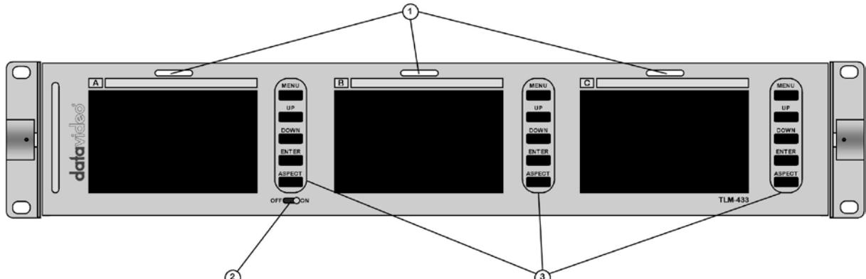
1. Each monitor has a bi-colour tally light indicator which can be connected to the Datavideo TB-10, or similar products. AMBER indicates Cued-Up and RED indicates Live (On-Air).
