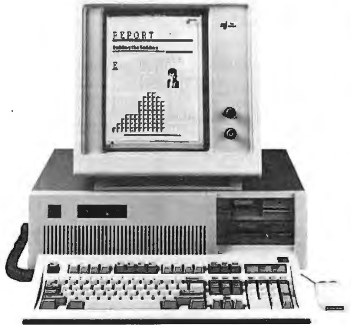
The Genius® Full-page Display: 66 lines in very high resolution - 100 dots/inch
