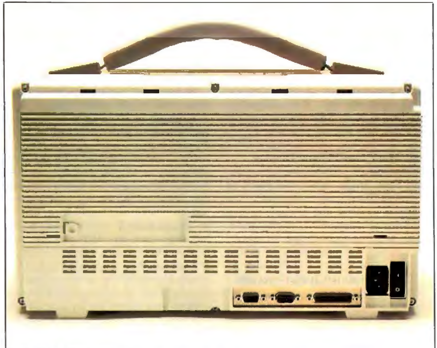
Photo 2: The rear view of the Portable III Model 20. Note the various ports, the sliding cover over the 96-pin port, and the machine's built-in padded handle.
