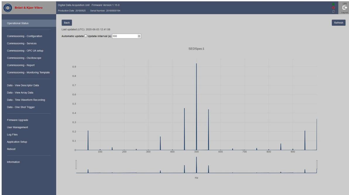
Figure 2 VCM-3 Homepage: Data – View Array Data (Example: FFT spectra derived from vibration velocity descriptor “BPI”)
