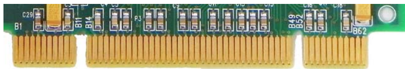
Supports both 3.3 V and 5 V PCI signaling environments
