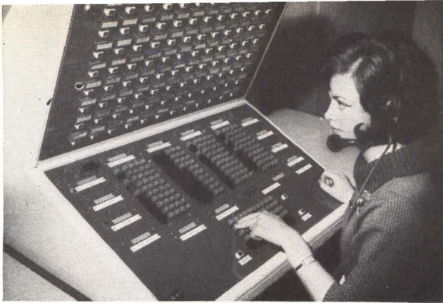
KEYBOARD of computer that simulates actions of 100 pilots is used in British atc experiments
