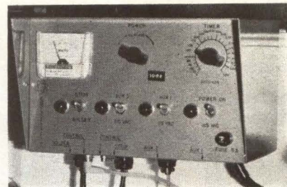
SOLID STATE supply provides adjustable current pulses to probe. A foot switch controls the supply but machine turns off at a predetermined time
