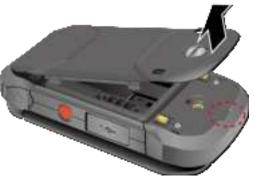
3. Insert the battery, making sure to align the gold contacts (1). Press down gently to secure the battery (2).
