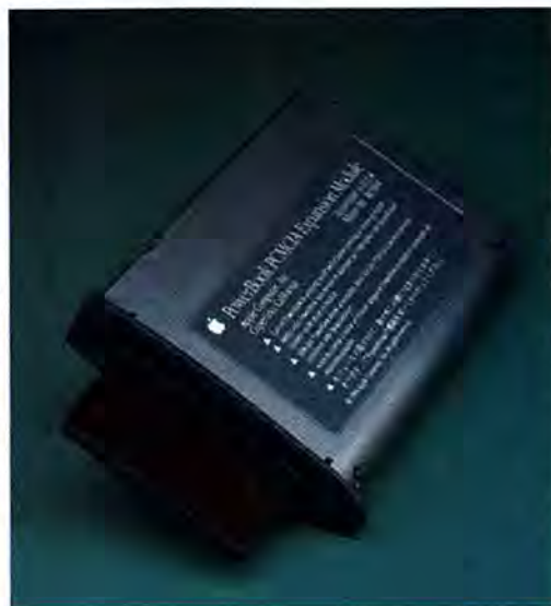
figure 1 / As small as a battery, Apple's PCMCIA expansion module fits in one of the two battery slots in a 500-series PowerBook and holds one Type III or two Type II PCMCIA cards. When Apple implements the PCMCIA Card and Socket Services standard, 500-series PowerBooks and Newtons will be able to use the same RAM, modem, wireless-network, and even hard-drive cards used in PC laptops. The credit-card-sized cards can be hot-swapped — that is, you can remove or replace them without having to reboot the computer.
