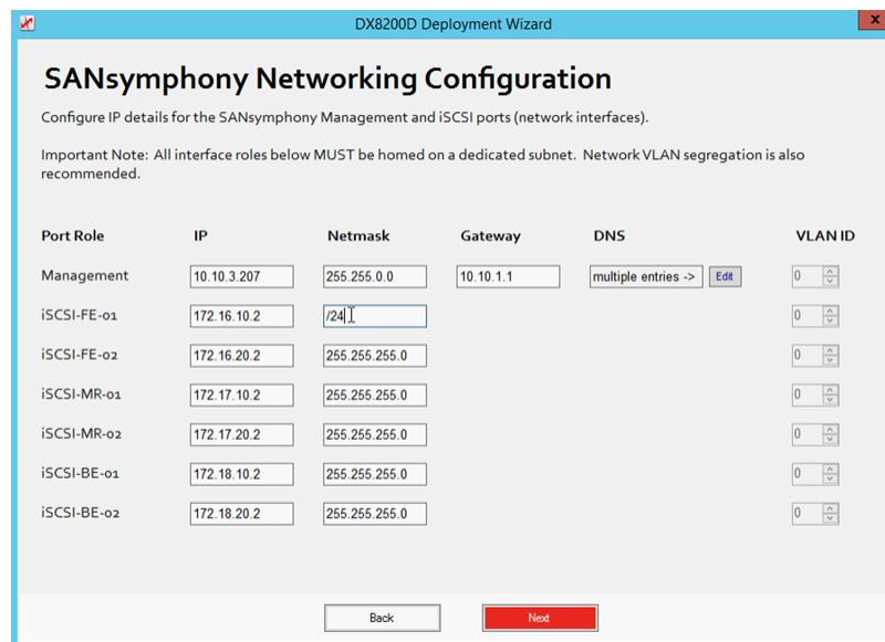
Correct operation of the SANsymphony™ software requires that all designated port roles (target or "Front-End" ports 'FE', storage "Mirror" ports 'MR', initiator or "Back-End" ports 'BE', and the out-of-band "Management" port) must be placed on separate logical networks. The GUI enforces this requirement and will display an error message if this constraint is violated. The deployment cannot continue until such an error is corrected:
