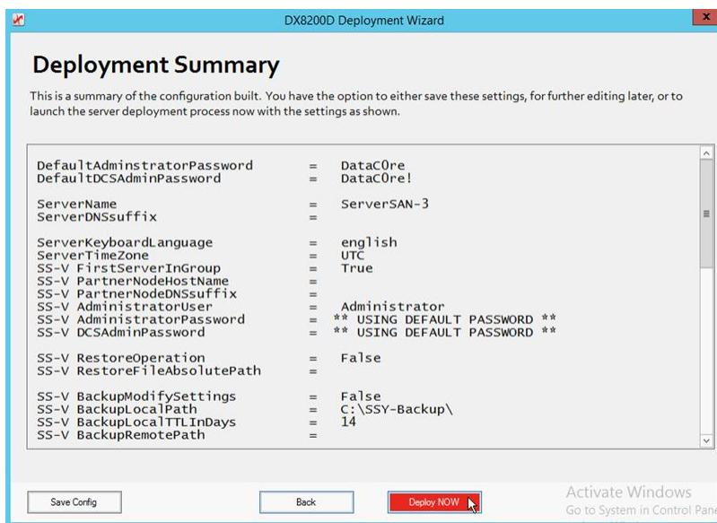
**Note:** For security reasons, when a configuration file is saved using the “Save Config” feature, any user supplied passwords will be removed and therefore will need to be re-input manually when the file is imported into another instance of the user interview GUI. This is because configuration settings are saved as plain text.
