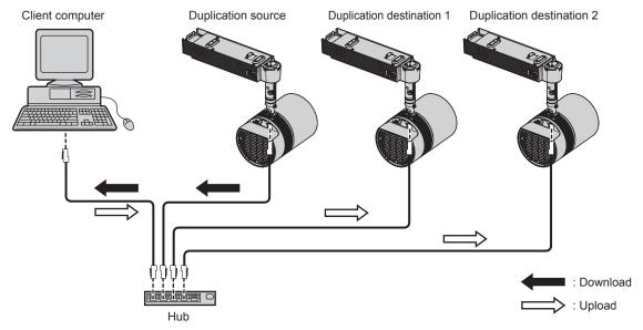
(Example) Illustration of connecting via wired LAN
