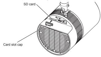
• Do not insert with excessive force when attaching the cap. Doing so may damage the terminal or the cap.
