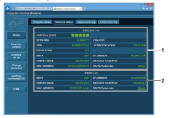
1 [WIRELESS LAN] Displays the settings of wireless LAN. 2 [WIRED LAN] Displays the settings of wired LAN.
