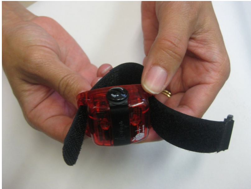
Figure 3-1. Threading the wrist strap through the PAM
