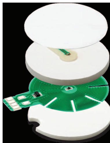
Figure 1. The SpotOn Prototype™ zero-heat-flux cutaneous thermometer. The cutaneous sensor consists of 2 thermometers, separated by an insulator, and covered by a heater. The heater is servocontrolled to keep the 2 temperatures identical. At that point, an isothermal tunnel develops below the skin surface so that surface temperature is about the same as subcutaneous temperature. In many parts of the body, subcutaneous temperature is similar to core temperature. Reproduced with permission © 3M 2013. All rights reserved.
