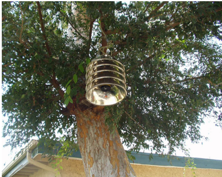
Photo 1 – Ambient H_2S - App-tek OdaLog
