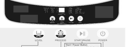
Powered on , press this button to launch machine .
