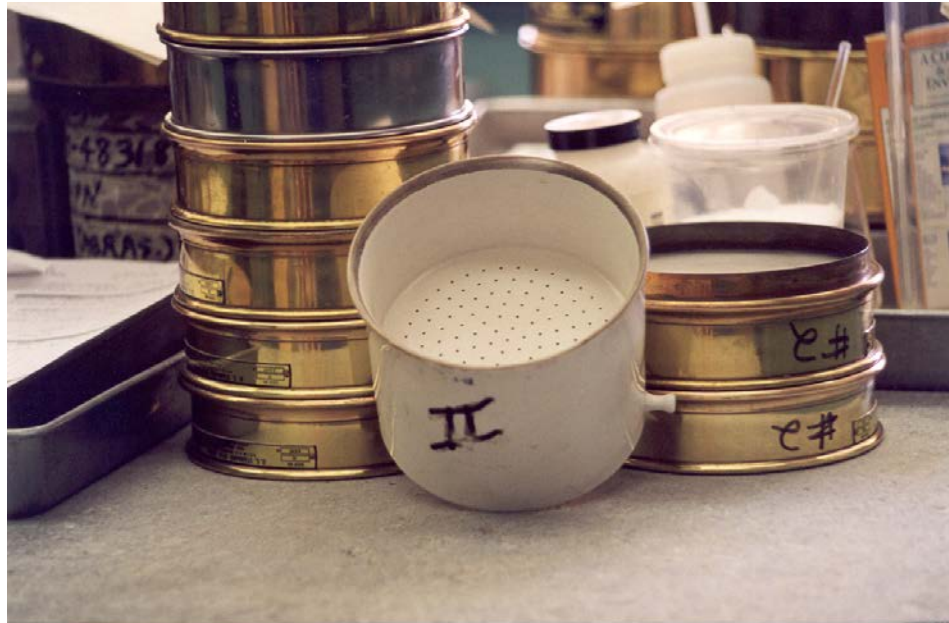
Figure 2- A porcelain Buechner funnel with a capacity of 750 mL and a plate with a diameter of 126 mm (5 inches).
