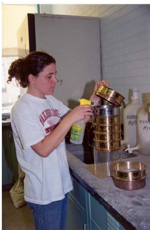
Figure 5- Spraying to clean off the interior of the sieve skirts
