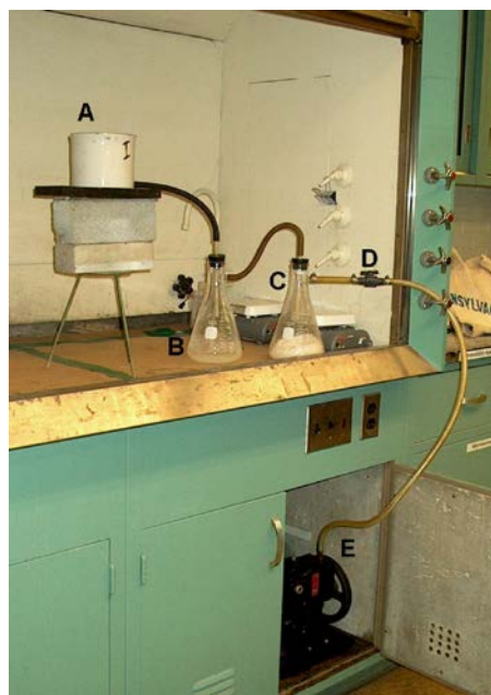
Figure 6- Vacuum set-up for the Buechner funnel A. Buechner funnel B. Decanting flask C. Calcium chloride flask D. ON-OFF valve E. Vacuum pump.
