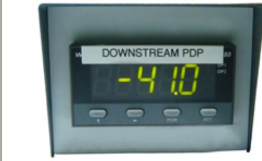
Example of a typical hygrometer using electrical sensing method based upon capacitance, resistance or conductivity
