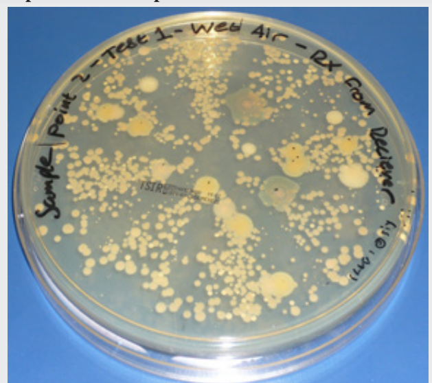
Agar plate with micro-biological growth from compressed air sample
