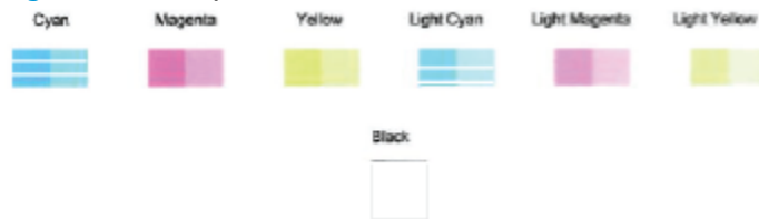
Figure 9-2 Example of color blocks with defects
